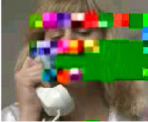
(a) PSNR = 14.09 dB E_S/N_I = 20 dB Uncoded
