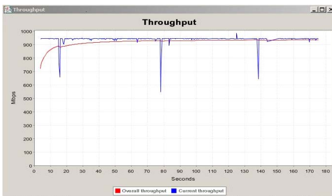
Fig. 6 – The throughput recorded for a 20 GB file transfer. The effective file transfer rate measured over OMNInet was 920 Mbps using ftp .
